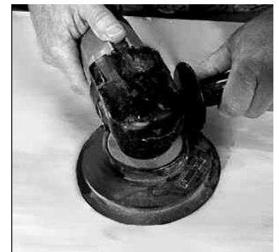
Fig. 23 Sanding using random Orbital sander
