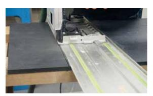
Using a biscuit jointer cut biscuit slots/ pockets to suit No.20 biscuits. Cut pockets 4mm down from the top face. Typically, 5 to 6 biscuits per joint minimum!
