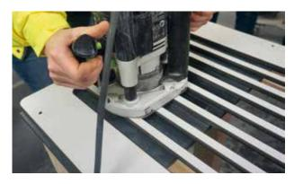
Please ensure the undermount sink inserts avoid the drainer groove positions, the inserts are designed to work in the entire thickness of the worktop.
