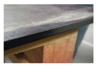
Image shows: Rough sawn edge, partially sanded.
