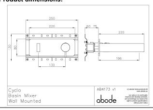
• Product mounted where: Wall • Recommended hole size: 200x60 mm
