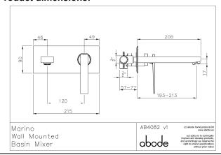
• Product mounted where: Wall • Recommended hole size: 195x70 mm
