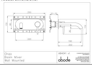
• Product mounted where: Wall • Recommended hole size: 188x58 mm
