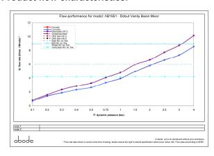
• Min / Max water pressure: 0.75 / 5.5 bar • Part G mixed flow rate at 3 bar (I/m): 8.72
