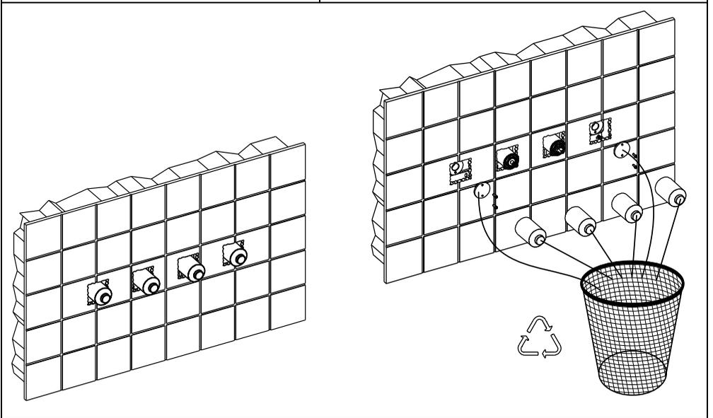
3. Discard plastic covers and brass water blockers as shown. **Note: Do not discard 4 x bolts.**
