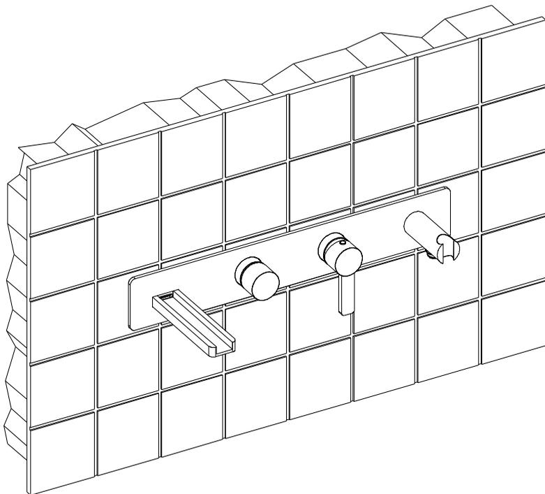
11. Apply clear silicone bead around the rear perimeter of the back plate (A).
