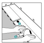
Always ensure that the short end joints will be staggered minimum 30 cm (= 3 click elements) when you start the next row. Use the leftover piece from the previous row as the first piece of the next row, provided that this piece is at least 30 cm. In order to find a connection with the locking tabs of the previous row, it may be necessary to cut off an extra part of the leftover piece.
