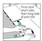
Always ensure that the short end joints will be staggered minimum 20 cm (= 2 click elements) when you start the next row. Use the leftover piece from the previous row as the first piece of the next row, provided that this piece is at least 20 cm. In order to find a connection with the locking tabs of the previous row, it may be necessary to cut off an extra part of the leftover piece.
