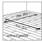
Measure the room to become a balanced lay out. By measuring, you will be able to determine if the first row needs to be cut. The first and last row should not be less than 5 cm wide.
