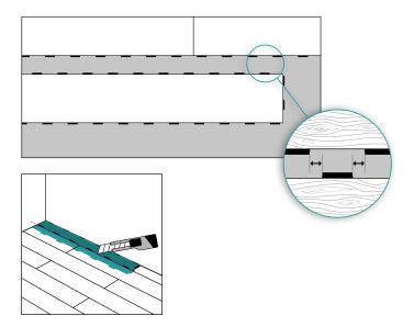
The click elements of the new row, need to be positioned, exactly in the middle of two locks of the previous row.
