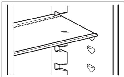
The walls of the refrigerator are equipped with a series of supports so that the shelves can be positioned as desired.
