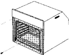
Secure the oven with 2 screws as illustrated.
