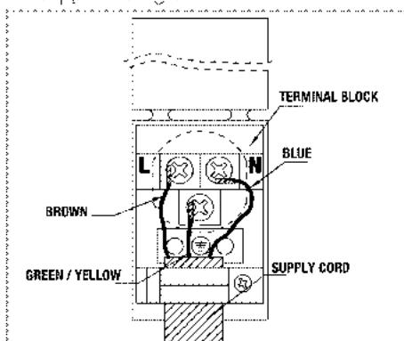
5. After completing the wire connections, close the terminal block cover.
