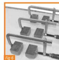
8. Adhesive excess must be removed at this stage from the joint before it hardens. Take care when doing so to ensure the joint remains fully closed. Adhesive overspill elsewhere on the surface may be wiped off using denatured alcohol. Go across the joint with a ruler or similar to feel if a step exists. If a step is found, then tap down until both sides are flat and level and re-tighten clamps. Ensure that you clean with denatured alcohol.
