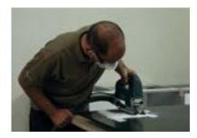
Set the pendulum setting on the jigsaw to '0' and the stroke rate to 1800spm. The key to jigsaw cutting M-Stone is patience: do not push the machine too hard, give the blade time to cut. Forcing the blade and pace will lead to blade defection and an out of square cut.
