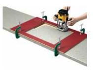
Using a 30mm guide bush and 1/2 inch router cutter, form a full depth cut-out, ensuring the waste section is supported to prevent damage as it falls away. Router cut in three stages of 15mm depth each. Remove the off cut and clean.
