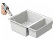
Adhesive will need to be applied to both worksurface cut-out and the mating flange of the sink. Due to limited workable time, adhesive application and assembly should be carried out speedily. Use adhesive that matches the worktop colour.
