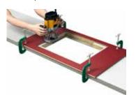
Accurately measure the total thickness of the worksurface and the jig. Accurately set the router cutter depth to the total thickness as measured less 4.5mm. Set and lock the depth stop.
