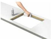
solid surface. Any dirt or dust trapped in the joint will compromise both mechanical and aesthetic quality of the seamless edge.
