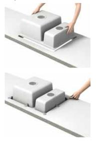
Refix the sink clips using the supplied screws. Evenly hand tighten the bolts and lock the nut ensuring you only tighten the bolts by hand. Tighten the lock nuts with a spanner.
