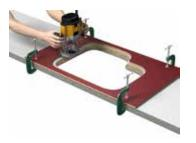
Waste removal has two stages using two different guide bushes:
