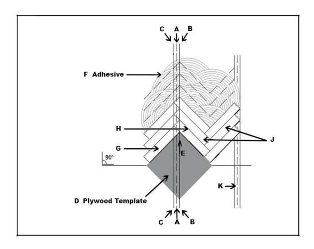
INSTALLATION OF HERRINGBONE ENGINEERED FLOORING
