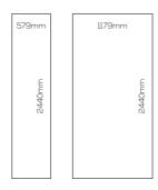
All Laminate panels are 10.5mm in thickness.
